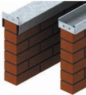
Multichannel brickwork restraints suit 100mm and 140mm block / brickwork walls and are available in lengths up to 9m either as a single or compound section. Attachment to the brickwork can be Rawlbolts (or similar), threaded rods built into the wall or flat strapped brick restraints built into the brickwork.
